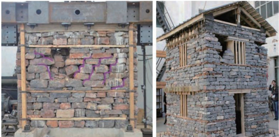
Figure 2-50: Set-up of house (stone, mud, with wood bands) being tested at Lab of Beijing Normal University. IRDR ICoE-NSET was one of the major collaborators. (Source: NSET (2017)).
